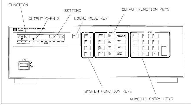
Figure 6-1. Front Panel (Model 6624A shown)
